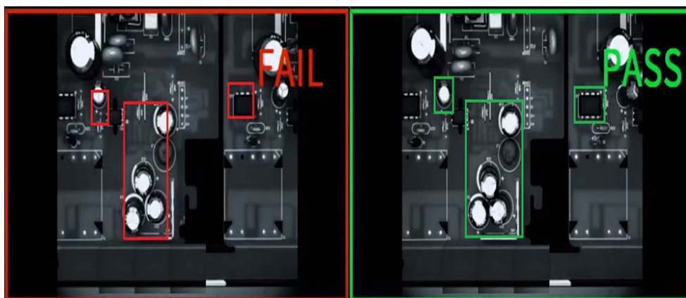
Fig. 2. Quality control according to the specified parameters
